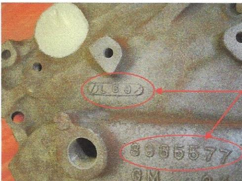
Intake manifold part # 3965577 is correct for L48 Engine.
