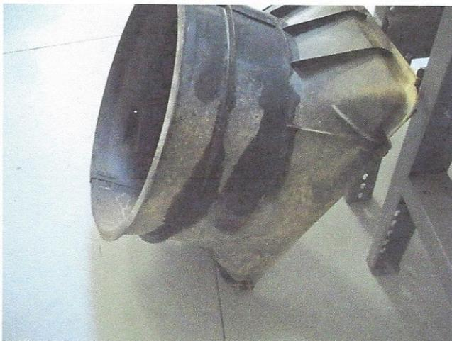
The fan shroud was removed and cleaned and repainted before installation.
